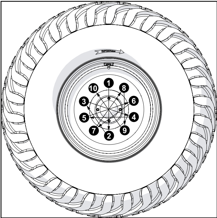
Fig. # 5-4 Wheel Lug Tightening Sequence (Diagonal Pattern)
