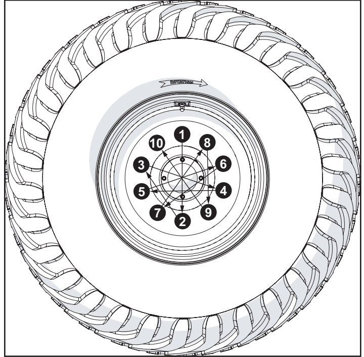
Fig. # 5-4 Wheel Flange Nut Tightening Sequence (Diagonal Pattern)
