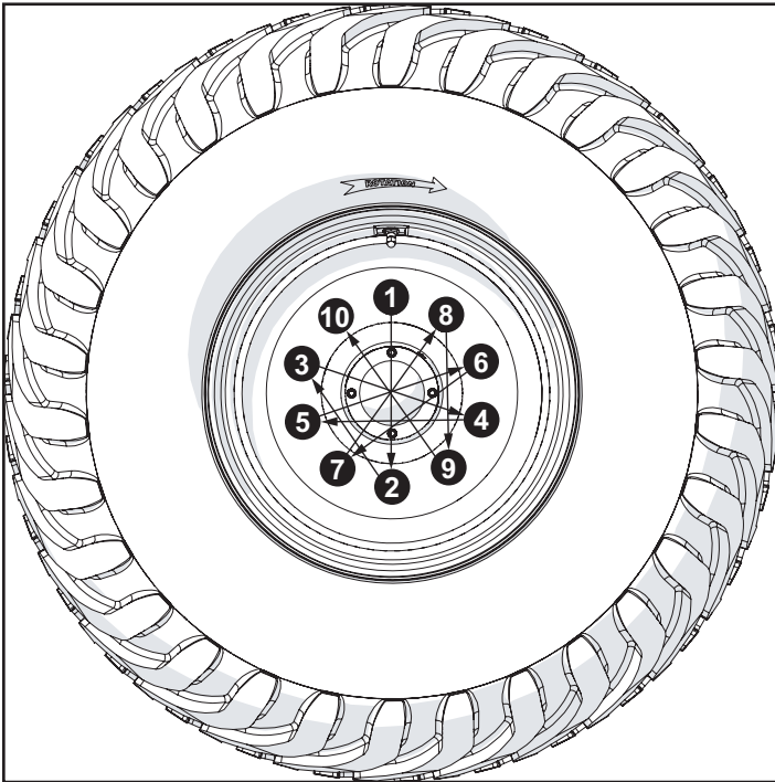
Fig. # 5-75 Wheel Flange Nut Tightening Sequence (Diagonal Pattern)
