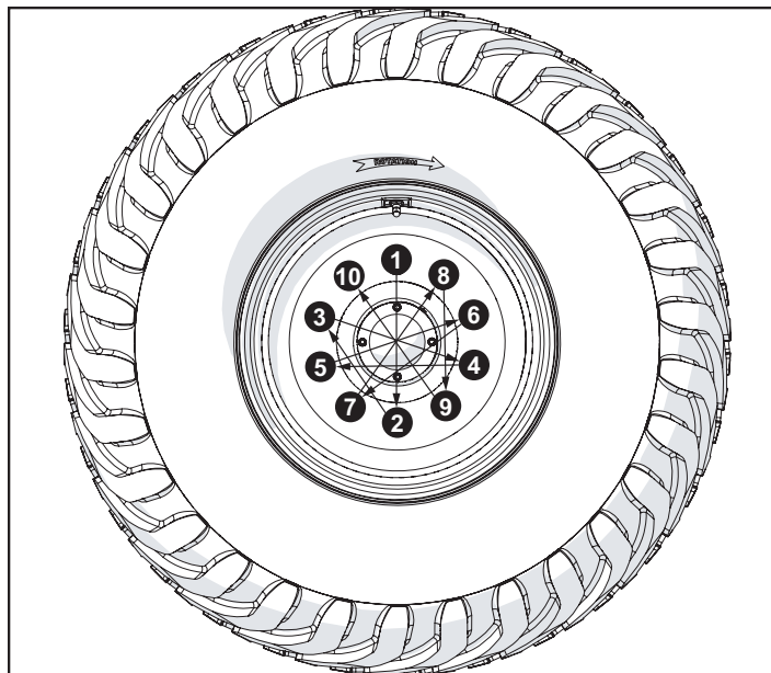
Fig. # 3-57 Wheel Flange Nut Tightening Sequence (Diagonal Pattern)
