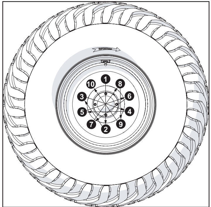
Fig. # 5-27 Wheel Flange Nut Tightening Sequence (Diagonal Pattern)
