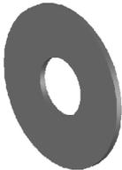
The pivot wear washer is used to prevent metal-to-metal contact of the suspension beam and the inside of the hanger. These wear washers can cup and misshape and still function. At the point the wear washer is worn thru, they should be replaced to prolong the life of the suspension.
