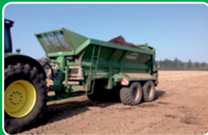
LOWLANDER WIDEBODY 230 HBD with built in flared extension sides, guillotine slurry door, sprung drawbar, weigh cells and 600/55 R26.5 tires.
