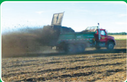
LOWLANDER 140 WIDEBODY TRUCK MOUNT with guillotine slurry door.
