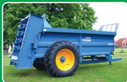
LOWLANDER 120 with guillotine slurry door.
