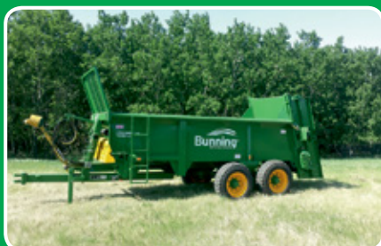
FARMSTAR 80 TANDEM with guillotine slurry door.
