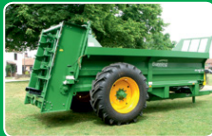
LOWLANDER 90 with guillotine slurry door.
