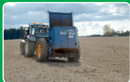
FARMSTAR 60 with guillotine slurry door and simple canopy spreading chicken litter.
