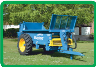
FARMSTAR 60 with guillotine slurry door
