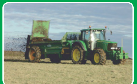
LOWLANDER 90 with guillotine slurry door.
