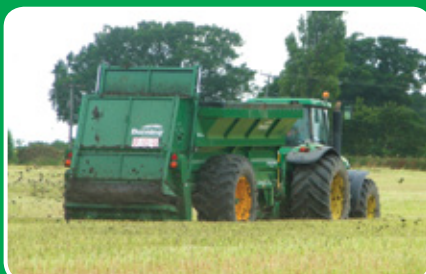
LOWLANDER 180 WIDEBODY HBD with 2 horizontal beaters and spinning discs, weigh cells, bolt on flared extension sides and 710/70 R38 tires.
