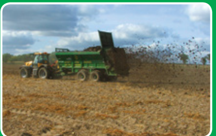
LOWLANDER 230 WIDEBODY sludge cake build with built in flared extension sides, wheels under body, and guillotine slurry door.
