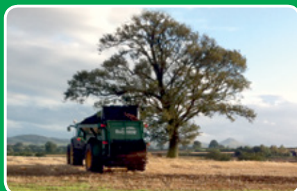
LOWLANDER 150 with 2 horizontal beaters and spinning discs, weigh cells, built in flared extension sides, guillotine slurry door and sprung drawbar.
