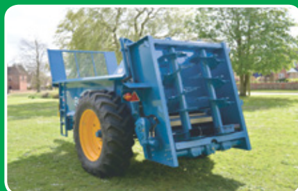
FARMSTAR 60 with guillotine slurry door.
