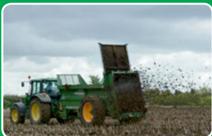
LOWLANDER 105 with guillotine slurry door.
