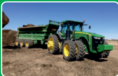
LOWLANDER 380HD with bolt on extension sides, guillotine slurry door, sprung drawbar and weigh cells.
