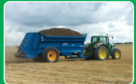
LOWLANDER 150 with detachable spinner deck, weigh cells, bolt on extension sides, guillotine slurry door and sprung drawbar.
