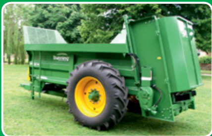
LOWLANDER 75 with guillotine slurry door and simple canopy.
