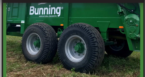
Tandem axle with sprung suspension
