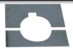
**Bin wall plates** seal the area where the unload tube exits the bin wall. The top half overlaps the bottom half by 1/2" for proper water shed. Manufactured from heavy duty galvanized steel.
