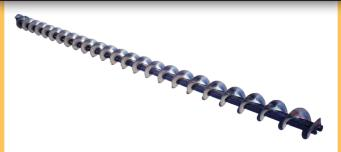
**Unload auger flighting** is manufactured from high quality mild steel components. Design is right hand full pitch, standard welds. All unload auger flighting is cut-to-length at the factory and are ready to be installed. Left hand pitch and brush flighting is available.
