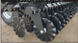
Four rubber elements provide a pretension, allowing the discs to follow the contour of the land. Skating over obstructions and springing back to operating position. Each shank is independent, allowing for ideal flow of residue.
