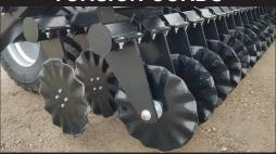
Four rubber elements provide a pretension, allowing the disks to follow the contour of the land. Skating over obstructions and springing back to operating position. Each shank is independent, allowing for ideal flow of residue.
