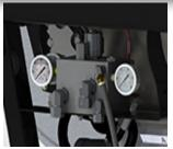
Pulse Width Modulation allows for control of the product metering system and the fan with only one hydraulic SCV required. The block includes safety valves to protect the fan seals and reduces heat in the hydraulic system.
