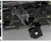
Eight individual High Density Polyethylene auger meters ensure proper metering of the commodity to the main hoses. Hoses can be split to achieve the desired distribution width from the deflectors.
