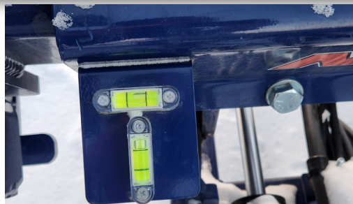
Ensures the mast is level to account for uneven terrain.
