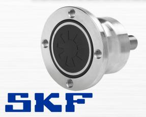
Relubrication-free: integrated solution increases farm productivity. Suitable for virtually any agricultural implement arm, the SKF Agri Hub for tillage discs is a robust, easy fit hub sealing solution. The unit features a flanged outer ring that is predrilled and tapped to accommodate a disc. A stationary inner ring fitted with a threaded stub shaft helps ensure fast, easy mounting.
