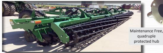
**CAGE ROLLER (standard)**: works best in dry, non-sticky soil conditions. The cage design ensures disintegration of any clumps, provides an even seedbed and moderate compaction.
