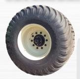
Unsurpassed flotation that has a large contact area. Makes for excellent weight distribution for reduced ground-bearing pressure and less soil compaction.
