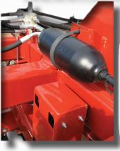
The accumulator is used in conjuction with a cross over relief valve to protect the wing cylinders from damage. Helps prevent damage by overextending cylinders or if the float position is forgotten to be put in place before use.
