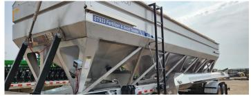
Allows user a safe way to climb to view the top of the tender.
