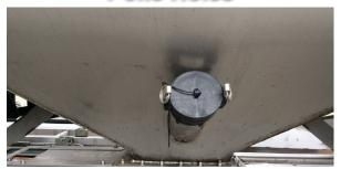
Allows user the ability to break up settled commodity for continuous conveyor flow.
