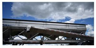
The belt return is enclosed to ensure safety and longevity.
