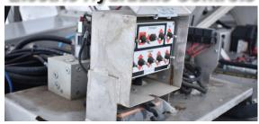
Controls gates and conveyor. Includes electronic override control box. Cased in a weather-proof stainless steel box.
