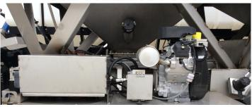
Self-contained hydraulic power pack, includes a 38HP Kohler EFI engine, pump and reservoir. Integrated trailer houses two 25-gallon stainless steel tanks for hydraulic fluid and gasoline.
