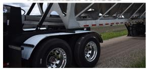
Aluminum wheels are corrosion resistant and lightweight.
