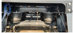
Only standard for ST900, ST933 and ST1166. Air ride system quickly adapts to the load of the trailer and road conditions.
